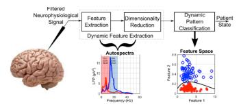
Fig. 1. Typical bio-signal processing chain of PD state determination during on-demand DBS.
