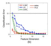
Fig. 7. Effect of feature vector dimension on classification error using: (a) DWT (b) STFT. The plots with the dashed lines are those using PCA for DR, while those without dashes use MRM for DR. The goal is to determine the minimum number of features that achieve a classification accuracy of 90% (10% classification error).
