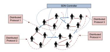
Fig. 2: Example of clustering for hybrid SDN control.
