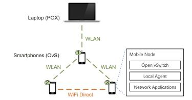
Fig. 5: The network topology involving three smartphones and the SDN controller installed on a laptop.
