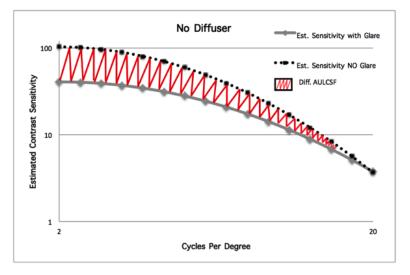
Figure 2. Difference of the area Under the Logarithmic values of CSF (Diff. AULCSF) from the measurement with the glare source on and off.
