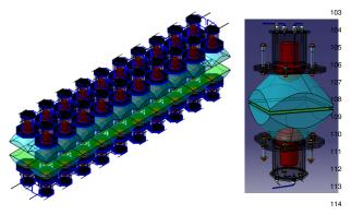
Figure 3: Details of the assembly of the 40 optical sub-modules inside a BiPo-3 module. On the right, a pair of optical sub-modules with the two thin scintillators (in green) face-to-face, coupled with a PMMA optical guide (blue) to a low radioactive 5 inches PMT (red).
