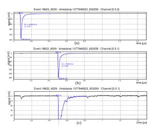
Figure 5: Display of a BiPo event identified as a bulk contamination inside the scintillators, with a signal in coincidence with the prompt signal in the opposite scintillator: (a) the prompt signal, (b) the delayed signal, (c) a zoom of the delayed signal with the coincidence signal. Using the coincidence of the prompt signals, these kind of background events are rejected.
