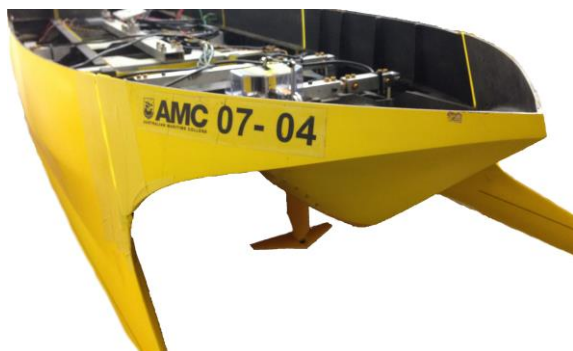
Figure 5: T-Foil installed on the aft section of the centre bow in a similar configuration to the full-scale INCAT 112 m vessel.
