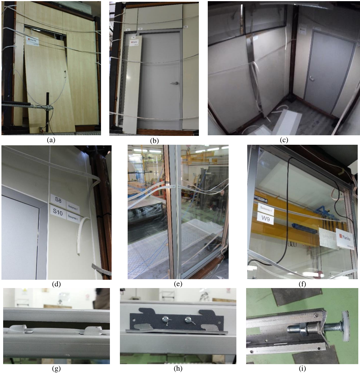
Figure 16. Recorded damages: (a) detachment and fall of Classic panels, (b) P85 panels, (c) Steel panels; (d) detachment of the flexible silicone-based material in P85 partition and (e) Glass partition; (f) detachment of the silicone-based material in glass panel; (g) deformed glass panel hooking system with steel frame and (h) with aluminum frame; (i) deformed P85 stud
