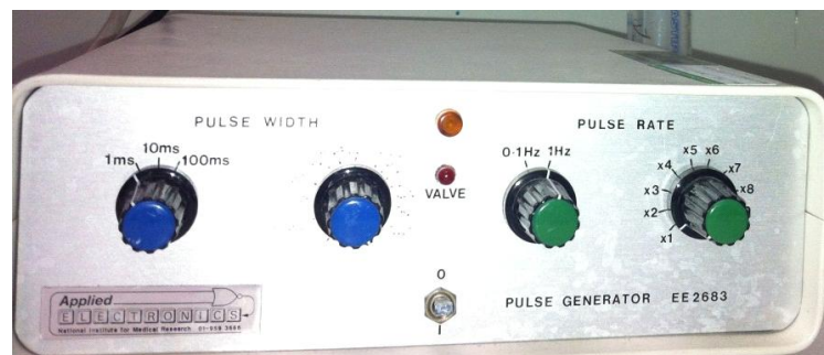
Figure10: After Applied electronic ltd, Uk “The width of the pressure pulses and the interval between them was controlled by pulse generator (Applied electronic ltd, Uk). These parameters were altered to suit variations in the cell suspension and in micropipette dimensions. Injection took approximately 4 min, commonly with a pulse length of 20 ms, a pulse interval of 1 ms and a delivery pressure of 20lbfjin. With such settings, slight downward movement of the meniscus could be observed with each pulse of air. Failure in meniscus movement was corrected by stepwise increase in pulse length or air pressure”.
