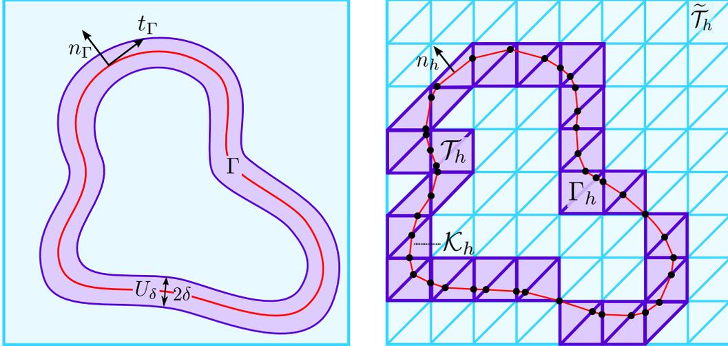
Figure 1: Set-up of the continuous and discrete domains. (Left) Continuous surface  $\Gamma$  enclosed by a  $\delta$  tubular neighborhood  $U_\delta(\Gamma)$ . (Right) Discrete surface  $\Gamma_h$  embedded into a background mesh  $\tilde{\mathcal{T}}_h$  from which the active (background) mesh  $\mathcal{T}_h$  is extracted.
