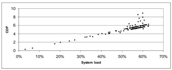
Figure 7: EER of Inverter Split System with System Load
