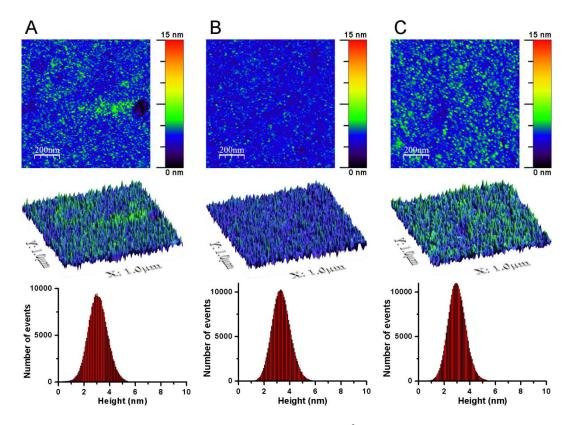
**Figure S2.** The first row contains AFM height images  $(1 \times 1 \ \mu m^2)$  of self-assembled PEI on silicon wafer at three different locations on the sample. The middle row presents AFM 3D images of the coatings (scale bar same as top row). The bottom row shows relative height histograms for AFM topographic images.
