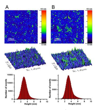
**Figure S4.** The first row contains AFM height images  $(1 \times 1 \ \mu m^2)$  of scans at two different locations on self-assembled and crosslinked PEI on silicon wafer after the  $10^{th}$  uptake cycle. The middle row presents AFM 3D images of the coatings (scale bar same as top row). The bottom row shows relative height histograms for AFM topographic images.
