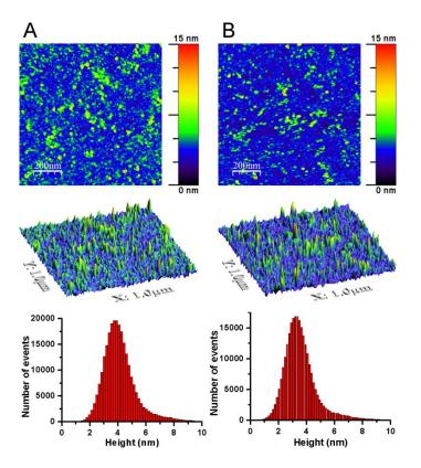
**Figure S5.** The first row contains AFM height images  $(1 \times 1 \ \mu m^2)$  of scans at two different locations on self-assembled and crosslinked PEI on silicon wafer after the  $10^{th}$  release cycle. The middle row presents AFM 3D images of the coatings (scale bar same as top row). The bottom row shows relative height histograms for AFM topographic images.
