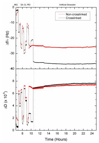
**Figure S6.** QCM-D sensogram of the stability of non-crosslinked and crosslinked self-assembled of PEI on silica-coated QCM sensors in artificial seawater. Normalized frequency (top panel) and dissipation change (bottom panel) for the 5<sup>th</sup> overtone (v = 5). The vertical dotted lines indicate the change of solution and the solutions are specified in-between the lines (MQ = MQ-water and SA CL PEI = self-assembly and crosslinking of PEI).
