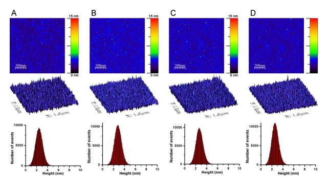
**Figure S1.** The first row contains AFM height images  $(1 \times 1 \ \mu m^2)$  of self-assembled PEI on silicon wafer at four different locations on the sample. The middle row presents AFM 3D images of the coatings (scale bar same as top row). The bottom row shows relative height histograms for AFM topographic images.
