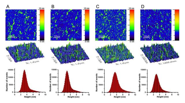
**Figure S3.** The first row contains AFM height images  $(1 \times 1 \ \mu m^2)$  of self-assembled and crosslinked PEI on silicon wafer. (A) and (B) represents scans at different locations on one sample and (C) and (D) represents scans at different locations on a different sample. The middle row presents AFM 3D images of the coatings (scale bar same as top row). The bottom row shows relative height histograms for AFM topographic images.
