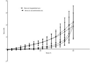
Fig 2:Stress-Strain graph for oesophageal specimens showing mean (kPa) and standard deviation
