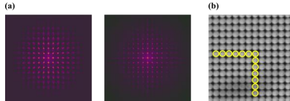
Fig. 2. (a) Magnitude of Fast Fourier Transform of a raw light field image of a uniform fluorescent layer captured before (left) and after (right) correction for pincushion / barrel distortion. (b) Corrected raw light field for a uniform fluorescent layer; yellow circles show experimentally determined size and pitch of pupil subimages.
