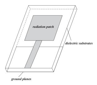
Figure 2. Structure chart of a printed monopole antenna.
