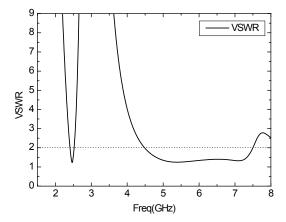
Figure 10. VSWR curve of the antenna.
