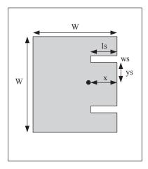
Figure 1. Structure of a microstrip antenna.
