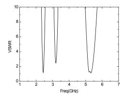
Figure 22. VSWR curve of the improved antenna.
