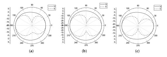
Figure 13. Antenna pattern (a) 2.45 GHz; (b) 5.2 GHz; (c) 5.8 GHz.
