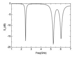
**Figure 18.**  $S_{11}$  parameter curve of the optimized antenna.
