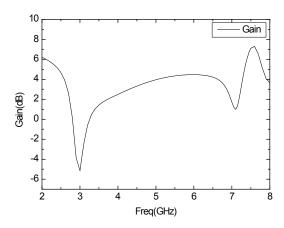
Figure 12. The gain curve of the antenna.
