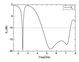
**Figure 9.** Parameter  $S_{11}$  of the antenna.
