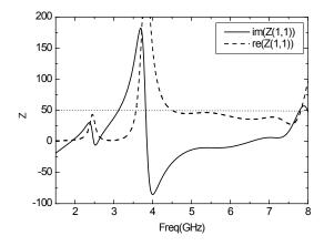
Figure 11. Input impedance curve of the antenna.
