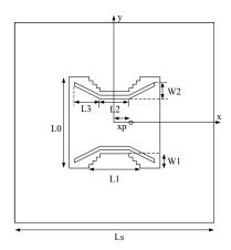
Figure 20. Improved antenna structure.
