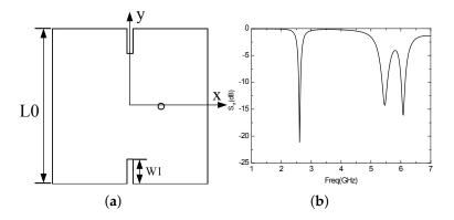
**Figure 16.** (a) Antenna structure with a rectangular slot; (b) The parameter  $S_{11}$  of the antenna with a rectangular slot.
