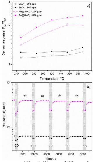
**Figure S3.** Sensor responses to 250 and 500 ppm of CO as a function of the operating temperature (a) and film-resistance changes towards 500 ppm of CO at 290 °C (b).
