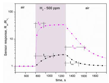
**Figure S4.** Normalised sensor response for 500 ppm of  $H_2$  (a) and CO (b) measured at 290 °C.  $t_R$  and  $t_{rec}$  represent the response and recovery time, respectively.
