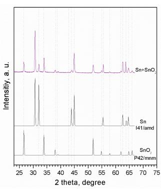
**Figure S1.** Typical XRD pattern of the aerosol assisted chemical vapor deposited films at 600 °C from methanol-based solution. The diffraction peaks in the data can be indexed to a tetragonal phase (P42/mnm) of tin oxide (ICCD card no. 041-1445) and a body-centered tetragonal phase (I41/amd) of metallic tin (ICCD card no. 004-0673)
