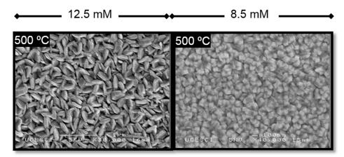
20 **Figure S2.** SEM imaging of the films deposited at 500 C from a methanol-based solution with different precursor concetration.
