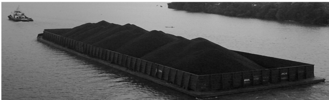
Figure 2: Coal transport operations utilize barges that carry up to 10,000 tonnes of coal.
