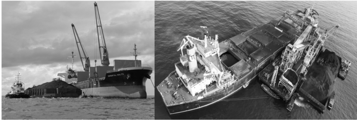
Figure 4: Barges are discharged onto ocean vessels using on-board (left) or floating cranes (right).
