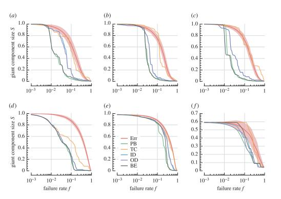
**Figure 6.** Robustness of the giant strongly connected component when each system is subject to five systematic attack strategies: TC, PB, BE, ID and OD. Vulnerability to random failure (Err) included for comparison. Shaded regions represent standard deviation (see figure 4 for standard error). (*a*) London Metro, (*b*) Paris Metro, (*c*) New York Metro, (*d*) US Flights, (*e*) C. Elegans and (*f*) StudentLife.
