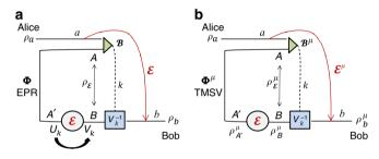
Figure 3 | Teleportation-covariant channels are Choi-stretchable.
