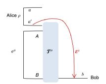
**Figure 9 | Asymptotic LOCC simulation of bosonic channels.** The finiteenergy LOCC simulation  $(\mathcal{T}^{\mu}, \sigma^{\mu})$  generates a teleportation channel  $\mathcal{E}^{\mu}$ . Assume that  $\mathcal{E}^{\mu}$  defines a target bosonic channel  $\mathcal{E}$  according to the pointwise limit in equation (93). Then, we say that the bosonic channel  $\mathcal{E}$ has asymptotic simulation  $(\mathcal{T}, \sigma) := \lim_{\mu} (\mathcal{T}^{\mu}, \sigma^{\mu})$ .
