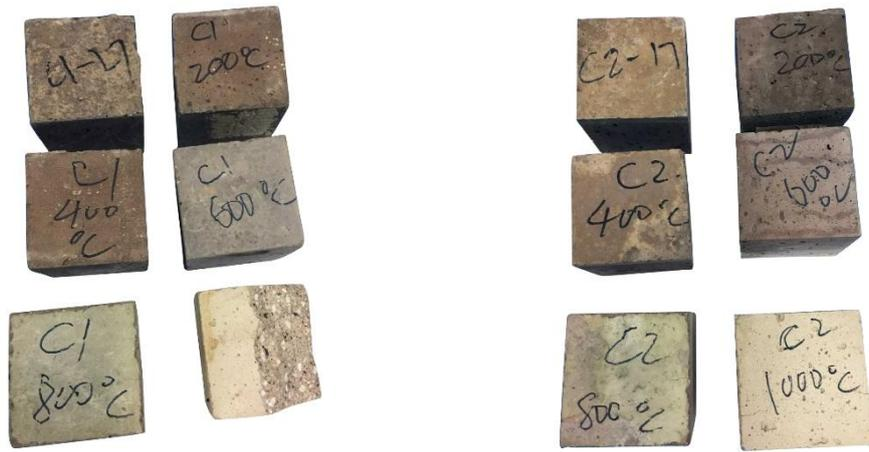
**Fig. 2.** Specimens (partial) before and after high temperatures treatment.
