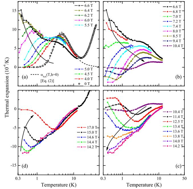
FIG. 2 (color online). Thermal expansion  $\alpha = 1/L \partial L / \partial T$  measured along the  $c^*$  direction in various magnetic fields (a) below  $H_{c1}$ , (b),(c) between  $H_{c1}$  and  $H_{c2}$ , and (d) above  $H_{c2}$ . Note the logarithmic temperature scale. The dashed line in (a) is a fit with the Schottky formula Eq. (2). The arrows signal the order of the  $\alpha(T)$  curves with increasing field.
