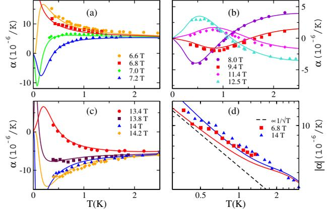
FIG. 4 (color online). Panels (a)–(c) compare representative experimental data (symbols) of  $\alpha(T)$  to theoretical curves (lines) obtained within the free-fermion model (4). All these curves are fully determined by  $H_{c1/c2}$  and a factor  $\gamma$  obtained from a fit to  $\varepsilon(H)$  data at  $T = 335$  mK (see Fig. 1). Panel (d) shows the thermal expansion near  $H_{c1/c2}$  on a double-logarithmic scale together with the limiting  $1/\sqrt{T}$  behavior (dashed line).
