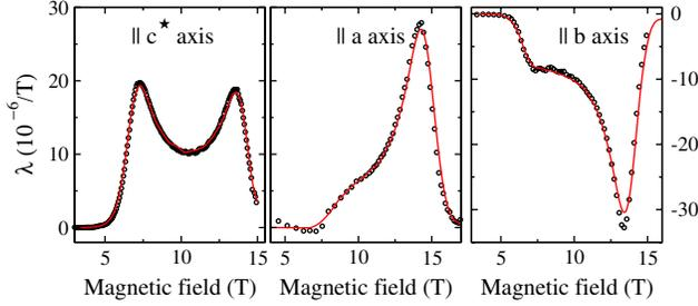
FIG. 5 (color online). Anisotropic magnetostriction coefficients  $\lambda$  (symbols) measured along  $c^*$ ,  $a$ , and  $b$ . The lines are quantum Monte Carlo fits using the experimental values of  $J_{\perp}$  and  $J_{\parallel}$  and two additional parameters for each direction, which measure the uniaxial pressure dependencies of  $J_{\perp}$  and  $J_{\parallel}$  [22].
