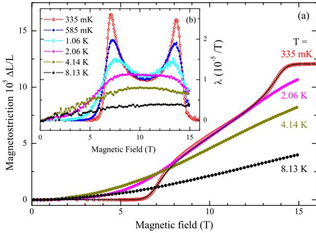
FIG. 1 (color online). (a) Magnetostriction  $\varepsilon = \Delta L(H)/L$  and (b)  $\lambda = \partial\varepsilon/\partial H$  measured along  $c^*$ . The solid line in (a) is a fit of  $\varepsilon$  at 335 mK within a free-fermion model.
