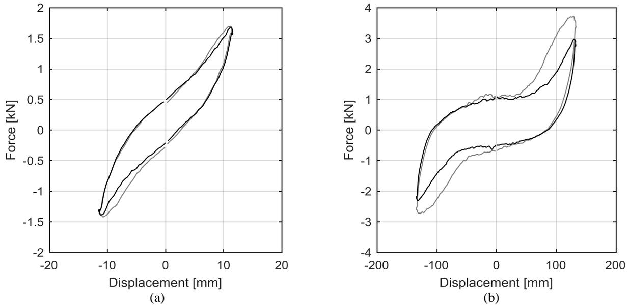
267 **Figure 11. Force-displacement relationship for (a) step no. 9 and (b) step no. 16 of the defined loading test**
