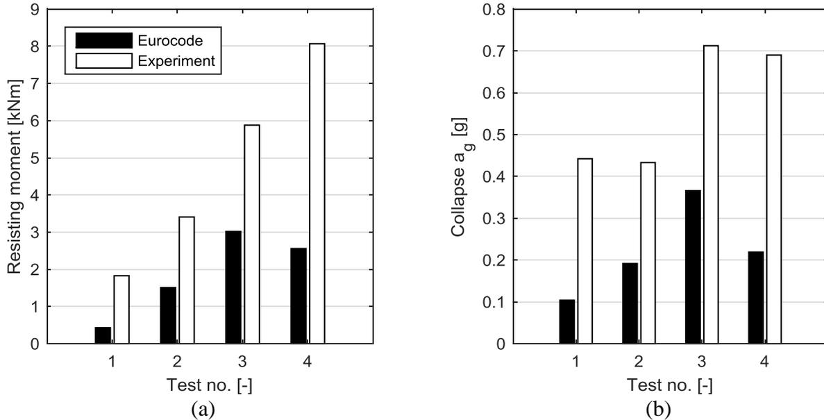
421 **Figure 17. Comparison between (a) resisting bending moments and (b) collapse ground accelerations evaluated**
