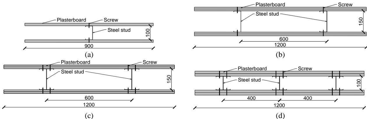
153 **Figure 4. Test specimen cross-sections: (a) specimens no. 1, (b) specimen no. 2, (c) specimen no. 3 and**
