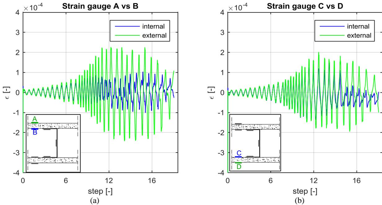
301 **Figure 14. Strain gauge recording in both the sides of the two plasterboards installed in specimen no. 1.**
