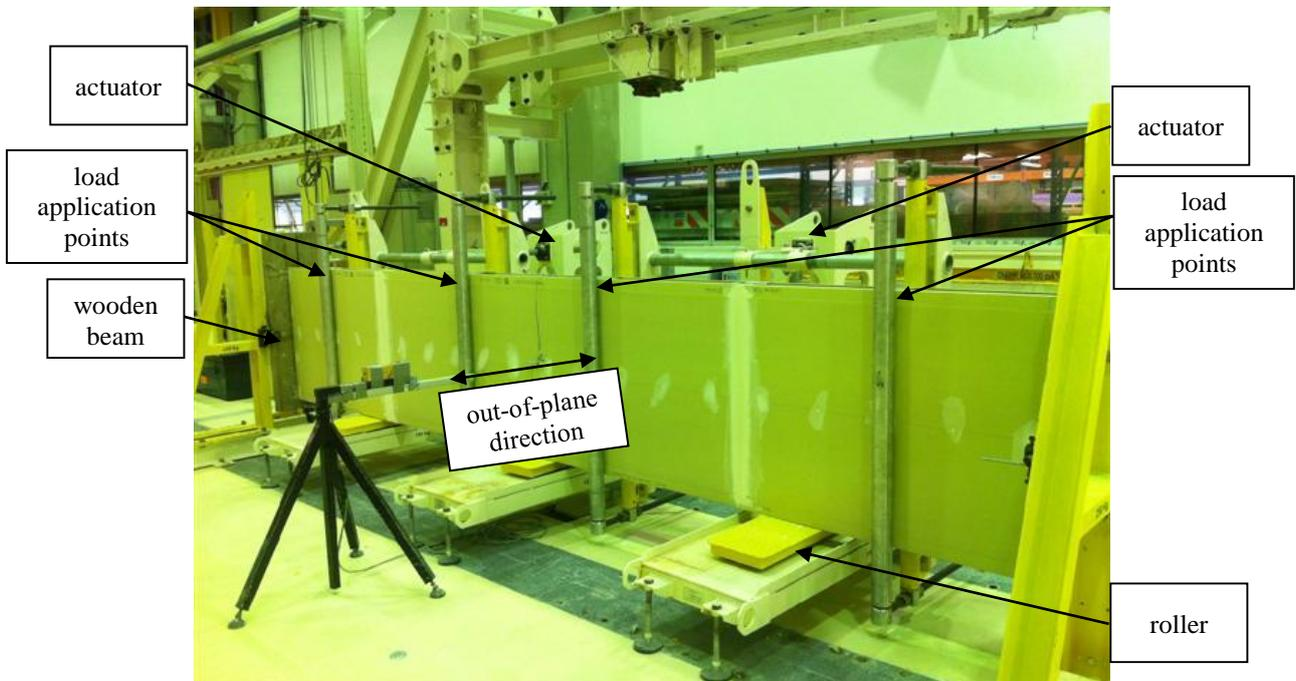
101 **Figure 1. Global view of the test setup for specimen no. 1.**
