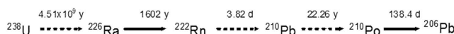
Figure 2. ^{238}\text{U} decay series, showing the principal radionuclides concerned with the production of ^{210}\text{Pb} and their radioactive half-lives. (Dashed arrows indicate decay through one or more intermediate radionuclides).
