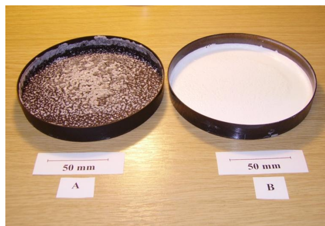
Figure 3. Unfoamed evaporated sea-salt solution ( 35 \text{ gL}^{-1} ) (A) without additives and (B) with 0.5 wt.% HPMC (Methocel™ E50). The dishes were polystyrene Petri dishes of 135 mm diameter sprayed with matt black paint. They were filled to a height of 15 mm giving 0.53 \text{ kg m}^{-2} salt residue. The reflectance measurements are given in Table 2.
