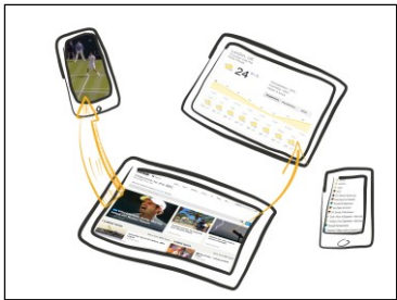
Figure 3: Content can be distributed across multiple devices (here: content can be flicked between two tablets and two phones). Device's position and orientation is tracked using HuddleLamp, allowing for a shared canvas and cross-device interactions.
