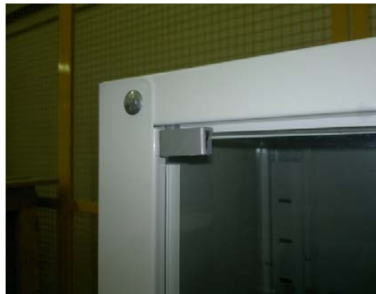
332 333 Fig. 11. Connection between the steel elements and the glass window of the single-window cabinet.
