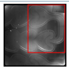
**Figure 3.** Example image acquired by the PIV camera (frame A) indicating the region of interest (ROI), shown by the red rectangle, which was located at the last heart cell of row 4 and the first heart cell of row 5.
