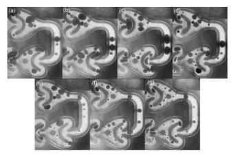
**Figure 13.** Bubble distributions in the region of interest for a gas volume transport fraction of  $\beta$  = 0.25 at different overall flow rates: (a) 10 mL/min; (b) 15 mL/min; (c) 20 mL/min; (d) 25 mL/min; (e) 30 mL/min; (f) 35 mL/min; (g) 40 mL/min.
