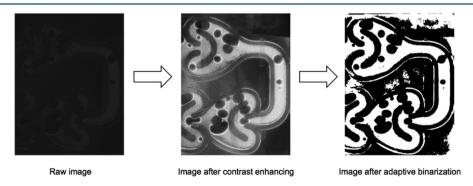
Figure 4. Schematic of the procedure for generation of the image mask.
