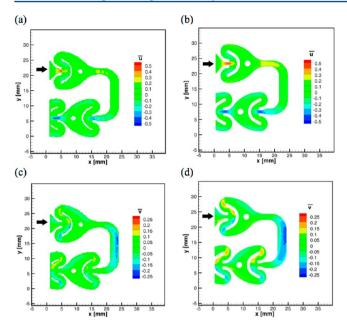
Figure 7. Comparison between PIV (left column) and CFD (right column) results for single-phase flow at a flow rate of 30 mL/min: (a)  $\overline{u}$  from PIV; (b)  $\overline{u}$  from CFD; (c)  $\overline{v}$  from PIV; (d)  $\overline{v}$  from CFD.
