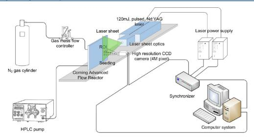
Figure 2. Schematic diagram of the experimental PIV setup.
