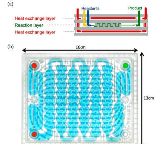
Figure 1. (a) Cross-sectional view of the Corning AFR module showing the two heat exchange layers and the reaction layer. (b) Top view of the Corning AFR module. The two inlets are marked in red and the outlet in green.
