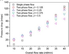
**Figure 17.** Experimental pressure drop results for single- and two-phase flow in the AFR: (a) pressure drop vs liquid phase flow rate; (b) pressure drop vs overall flow rate (gas and liquid phase).
