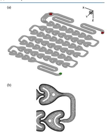
**Figure 6.** (a) Representation of the computational domain of the AFR used for CFD simulations. The inlets are marked in red and the outlet in green. (b) Computational grid for the ROI of the PIV measurements (last heart cell of row 4 and the first heart cell of row 5).
