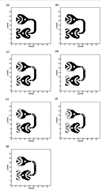
**Figure 15.** Ratios of the RMS velocity fluctuation magnitudes (two-phase flow/single-phase flow) for a gas volume transport fraction of  $\beta$  = 0.25 at different overall flow rates: (a) 10 mL/min; (b) 15 mL/min; (c) 20 mL/min; (d) 25 mL/min; (e) 30 mL/min; (f) 35 mL/min; (g) 40 mL/min. Dark regions indicate ratios larger than 1, and light regions indicate ratios smaller than 1.
