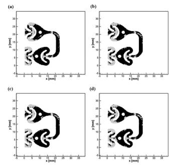
**Figure 12.** Plots of the ratio of the RMS velocity fluctuation magnitudes (two-phase flow/single-phase flow) for an overall flow rate of 30 mL/min: (a)  $\beta = 0.125$ ; (b)  $\beta = 0.25$ ; (c)  $\beta = 0.375$ ; (d)  $\beta = 0.50$ . Dark regions indicate ratios larger than 1, and light regions indicate ratios smaller than 1.
