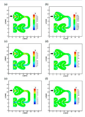
Figure 8. Mean velocity contours for single-phase flow: (a)  $\overline{u}$  for 10 mL/min; (b),  $\overline{v}$  for 10 mL/min; (c),  $\overline{u}$  for 25 mL/min; (d),  $\overline{v}$  for 25 mL/min; (e),  $\overline{u}$  for 40 mL/min; (f),  $\overline{v}$  for 40 mL/min.
