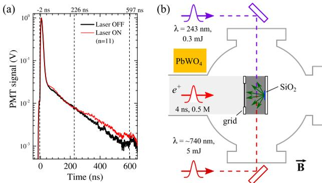
FIG. 1 (color online). (a) Example of single shot lifetime spectra with lasers on and off resonance as indicated, and (b) a schematic of the target chamber and Ps formation region. The time windows used to analyze the lifetime spectra are indicated by the dashed lines in (a). The shaded regions in (b) roughly correspond to annihilation times up to 226 ns (dark region) and later than 226 ns (light region).
