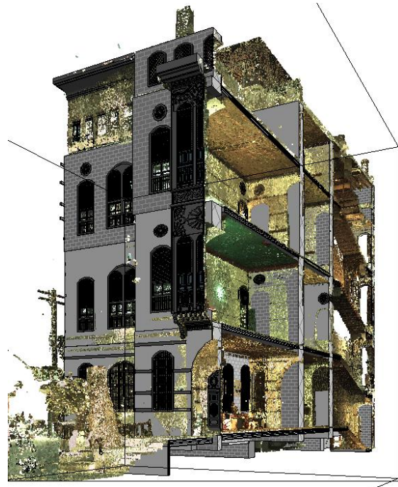
Figure 7: 3D section on the JHBIM model and the point cloud.
