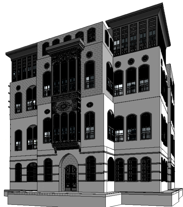
Figure 3: 3D model of Nasif Historical House based on JHBIM.
