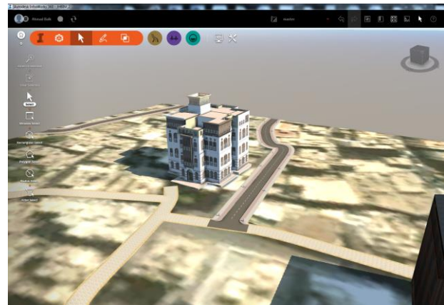
Figure 9: Integrating vector and raster data with the JHBIM of Nasif Historical House within Autodesk InfraWorks.
