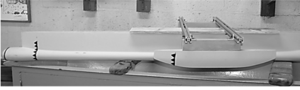
Figure 3. Tri-SWACH model used to obtain experimental towing tank resistance data (figure from [6]).
