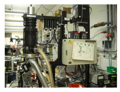
Figure 3.11 Seki technotron PECVD setup
