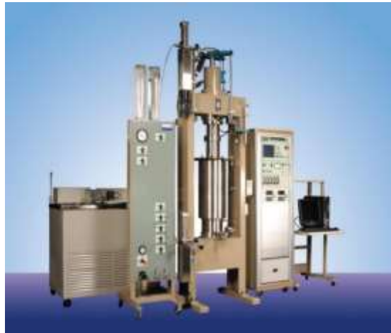
Figure 2.5: Methane hydrate soil experiment apparatus (Hyodo et al., 2011)
