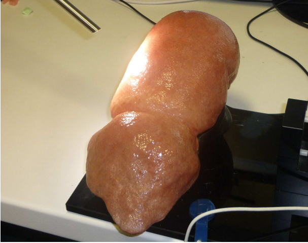
Figure 6. The silicone phantom mounted on the table in front of the stereo laparoscope. The visible part of the liver phantom is made of visually realistic flexible silicone
