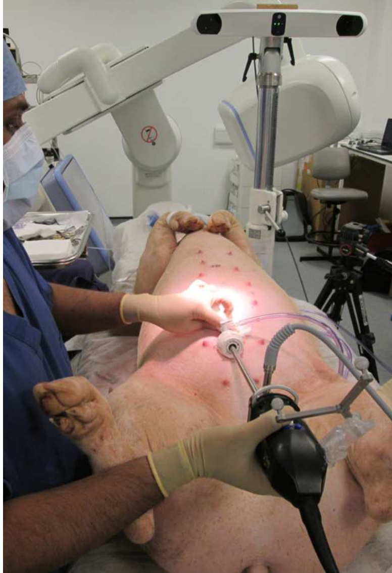
Figure 3. The optical tracking cameras, top right, track a rigid body of three infra red reflective spheres rigidly fixed to the external end of the laparoscope, bottom right.
