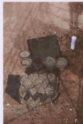
Fig. 107. Bulk fill, geo-drains and geotextile materials used for backfilling at Aztec (US01_0019).
