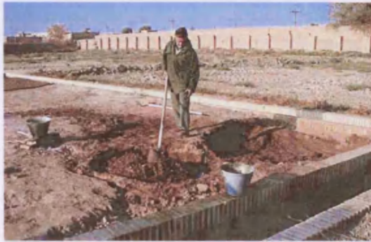
Fig. 7. General view of preparation of earth mix for mudbrick making, Yazd, Iran (IR07_0070).
