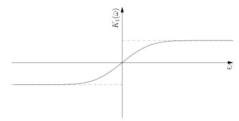
FIGURE 2. Graph of the function  $K_1(\bar{\omega})$  given by (84). This increases monotonically from -1 to +1 as  $\bar{\omega}$  increases from  $-\infty$  to  $+\infty$ .
