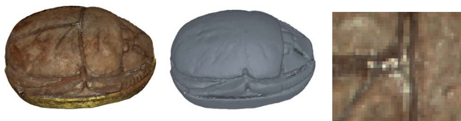
Fig. 5. (left) 3D reconstruction from the point cloud generated by the Arius laser scanner, showing the redness caused by the non-optimal laser wavelengths; (right) Detail of back.
