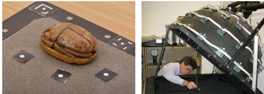
Fig. 2. (left) Photogrammetric imaging setup with scarab on target board; (right) positioning the scarab on the baseboard of the UCL dome.
