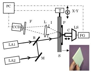
Fig.1 Experimental setup: LA1 – red laser; LA2 – green laser; B – dichroic filter ; M – mirror; I – iris; L – lens; S – scattering layer; P – color picture; C – connecting rod with a 2 mm screw at the tip; LS – loudspeaker; FG – function generator; F – Neutral density filter; CCD – CCD camera, T – 2-axes translation stage, PC – computer, and a photo of the scattering layer
