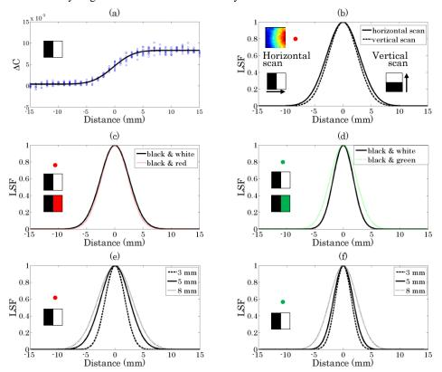
Fig. 3 Spatial resolution assessment: (a) the edge spread function, inset is the color picture hidden behind the scattering layer; (b) the line spread function (LSF) of the horizontal and vertical scans; the LSFs of the hidden pictures with different color combinations using (c) the red laser and (d) the green laser; the LSFs for different thicknesses of the scattering layers using (e) the red laser and (f) the green laser. (Insets are the hidden color pictures.)
