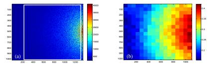
Fig.2 Speckle image: (a) the original speckle intensity image ( $1344 \times 1024$  pixels =  $4.3 \times 3.3$  mm), part of it (white box) cropped for analysis; (b) the cropped speckle contrast *C* (=  $\sigma / \langle I \rangle$ ) image ( $1100 \times 1024$  pixels =  $3.5 \times 3.3$  mm)
