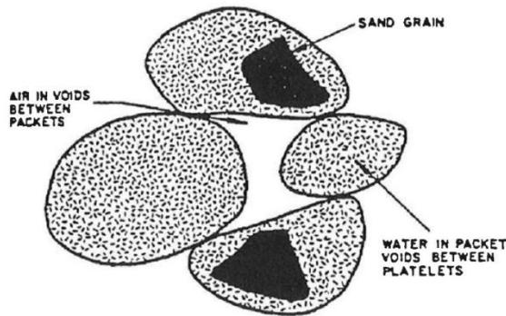
Figure 3: Model of unsaturated soil (Brackley, 1975)
