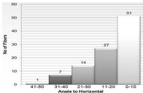
Figure 7: Alignment of fibres
