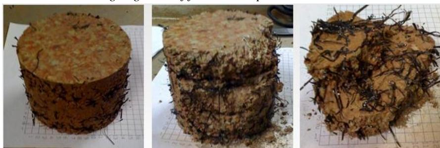
Photo3: Extruding fibres from sample
