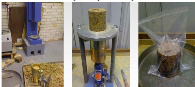
Photo 2: Reinforced sample compaction procedure
