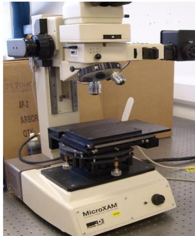
**Figure 3.21** ADE-MicroVAX light texture interferometer (picture by the author, 2011)
