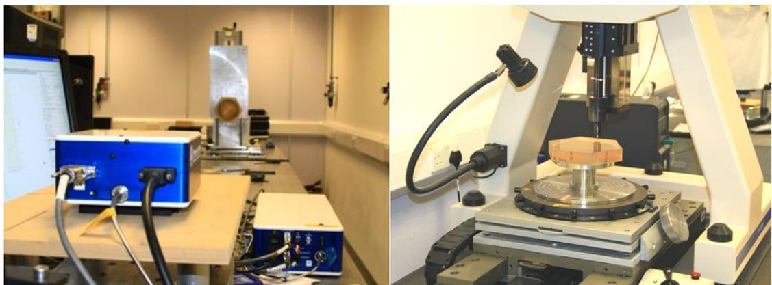
**Figure 6.7** The measurement set-up, where left is 4D interferometer, right is 'Extended Range' Form Talysurf (picture by author, 2011)
