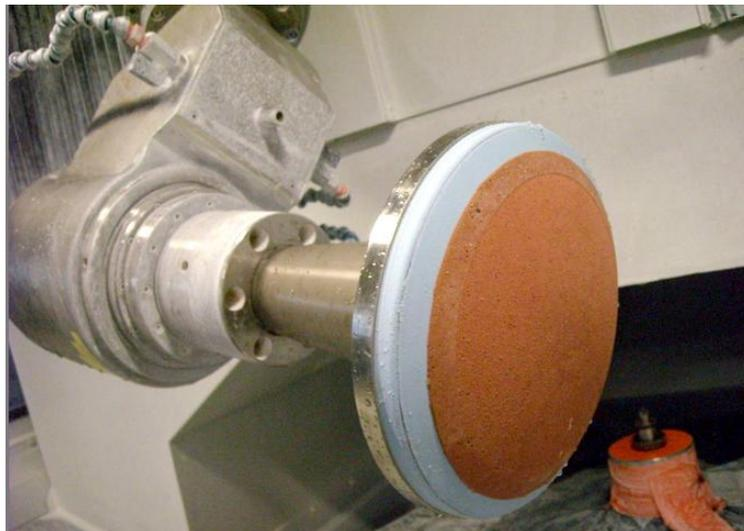
**Figure 8.4** New R200mm solid rubber tool with Polyurethane cloth on the IRP 1200 machine (author's picture, 2012)
