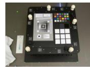
Figure 5. The completed 2D photographic target plate: Left ISO-16067-1 chart to test resolving power, top right: x-rite colour chart, bottom right: gloss scale.
