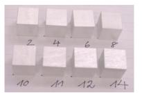
Figure 8. Test cubes after trial run for alkaline etching lined up for test 3D scan additionally to mechanical clocking.
