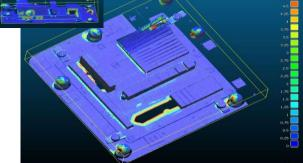
Figure 18 Comparison Arius3D scan vs Nikon MMD. Scale covers a +/- 0.5mm range and demonstrates systematic discrepancies between the two sets of measurement data. (Cloudcompare, http://www.danielgm.net/cc/)
