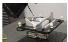
Figure 11. 3D colour laser scanning with an Arius3D Foundation system mounted on a Newport Goniometric Stage. The capabilities of the scanner are given in (Hess et al. 2011)(http://www.arius3d.com/a3d\_specs.html)
