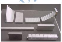
Figure 10. Mock-up for test scan before surface treatment: Angle artefact in two blocks, step artefact in two blocks. Length bars, gap artefact. Bottom left: gauge and does not belong to array.
