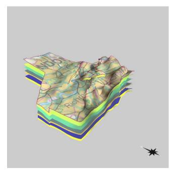
**Fig. 7.** 3D model of Chalk Group under London (Royse, 2010). OS data and Crown Copyright. All rights reserved. BGS 100017897/2011.
