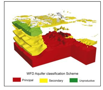
**Fig. 21.** Exploded volume model illustrating the Environment Agency's Water Framework Directive aquifer classification scheme for the East End of London. Adapted from Royse et al. (2009).
