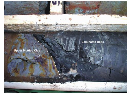
Fig. 8. Photograph of a Thames Water rotary core from the Stoke Newington area (north London) showing lower Woolwich Formation (Laminated Beds) faulted against upper Reading Formation (Upper Mottled Clay).
