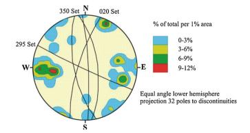
**Fig. 6.** Major persistent primary joints (many sheet-flint filled) and fault orientations in the Seaford Chalk Formation, Northfleet Quarries, north Kent. Adapted from Mortimore et al. (2011).
