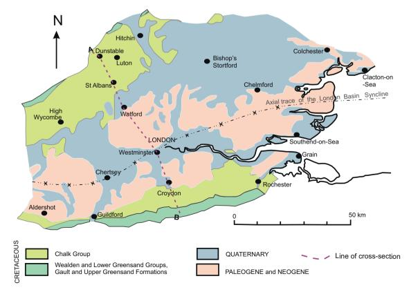
Fig. 1. Geological sketch map of the London Basin. Based on Sumbler (1996, Fig. 1).
