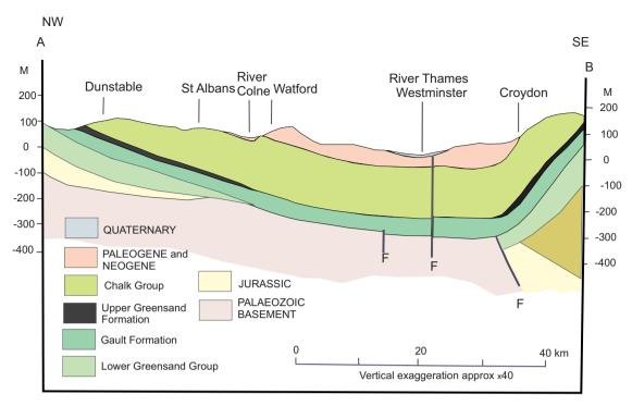
Fig. 3. Geological cross-section across the region showing the 'relatively simple' geological structure of region as previously proposed by Sumbler (1996). Section based on Sumbler (1996, Fig. 2).
