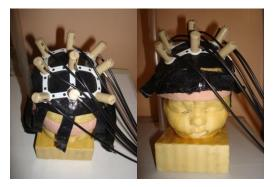
Figure 6.5: ETG-100 neonatal cap on dummy head.
