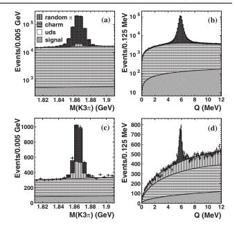
FIG. 2. Results of the M-Q fit for  $D^0 \to K^+\pi^-\pi^+\pi^-$ , in projections onto (a) RS  $M_{K3\pi}$  with 0 MeV < Q < 12.0 MeV; (b) RS Q with 1.810 GeV/ $c^2$  <  $M_{K3\pi}$  < 1.910 GeV/ $c^2$ ; (c) WS  $M_{K3\pi}$  with 5.47 MeV < Q < 6.28 MeV; and (d) WS Q with 1.852 GeV/ $c^2$  <  $M_{K3\pi}$  < 1.878 GeV/ $c^2$ .
