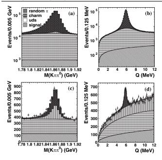
FIG. 1. Results of the M-Q fit for  $D^0 \to K^+\pi^-\pi^0$ , in projections onto (a) RS  $M_{K\pi\pi^0}$  with 0 MeV < Q < 12.0 MeV; (b) RS Q with 1.780 GeV/ $c^2$  <  $M_{K\pi\pi^0}$  < 1.920 GeV/ $c^2$ ; (c) WS  $M_{K\pi\pi^0}$  with 5.31 MeV < Q < 6.42 MeV; and (d) WS Q with 1.844 GeV/ $c^2$  <  $M_{K\pi\pi^0}$  < 1.887 GeV/ $c^2$ .
