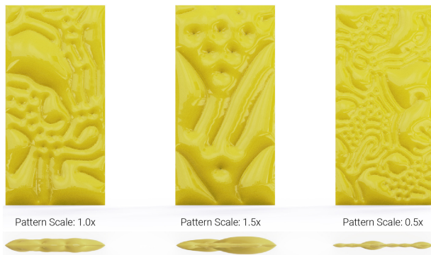
14 Relationship between the distance among point constraints and magnitude of inflation after thermoforming process.
