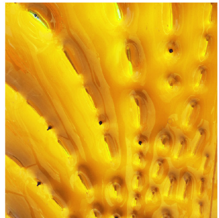
16 Multi-part assembled prototype of Variable Pneumatic Thermoforming (top right). Part-to-whole pattern composition of four individual unique panels. Varied visual aesthetics presented by the use of two color of PETG sheets; frontal opaque view (top left) and back transparent effects (bottom right).
