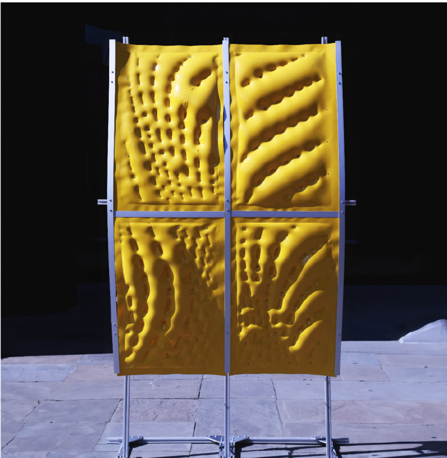
16 Multi-part assembled prototype of Variable Pneumatic Thermoforming (top right). Part-to-whole pattern composition of four individual unique panels. Varied visual aesthetics presented by the use of two color of PETG sheets; frontal opaque view (top left) and back transparent effects (bottom right).
