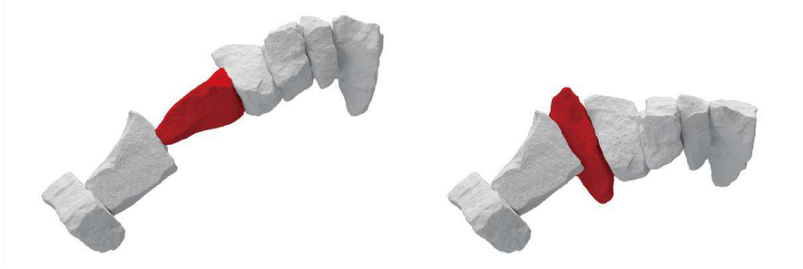
Figure 6. (a) The structure without area filtering exhibits a tiptoe-like stance, which is unstable. (b) After removing smaller-area faces, the aggregation shows improved structural stability.
