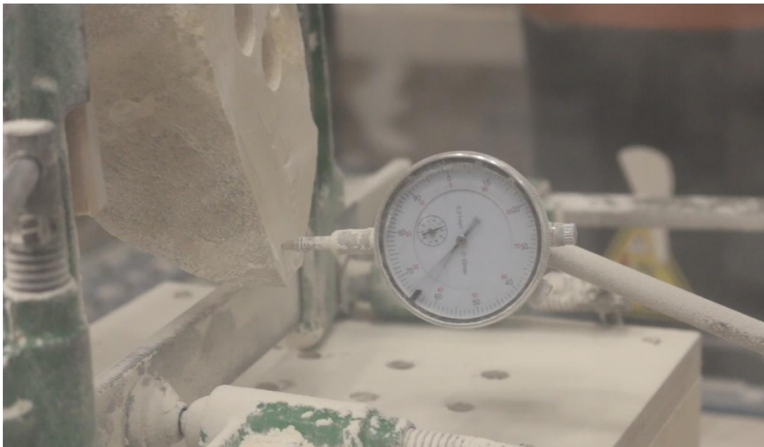
Figure 17. The pressure gauge could be used to detect the displacement.
