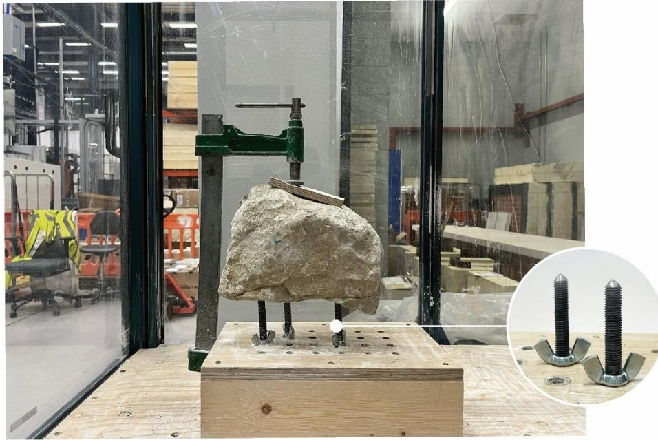
Figure 15. The modular work holding solution for irregular stones.
