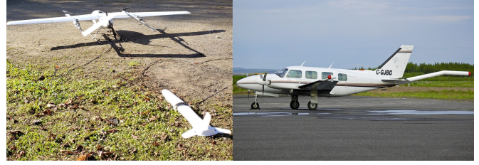
Fig. 5: (left) VTOL Fixed-wing UAV (SuMag; Suspended Magnetometer) with towed bird style magnetometer, in this case, a Geometrics MagArrow, and (right) fixed-wing crewed aircraft (Piper) with rear mounted stinger magnetometer, image from [47].
