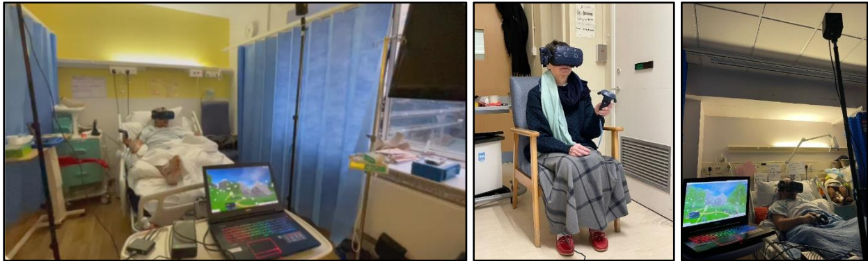
Figure 15: The ATTEND VR set-up on the ward. Components visible here are the 2 base stations on the tripods, the HTC Vive Headset as worn by the patients, the handheld HTC remote, the MSI Titan Pro laptop and hardware connections
