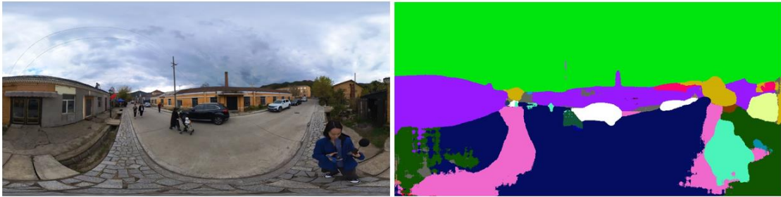
Fig.5 Semantic segmentation of 360 street image (use case 1 as an example)
