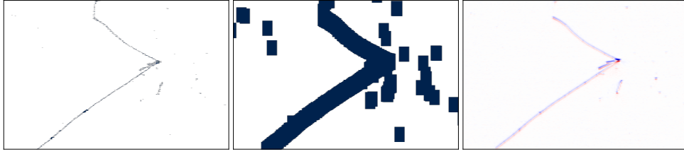
Figure 8.14: An example ND image (left), the associated signal mask (middle), and the associated FD image (right). Shown for a crop of near-far pair of the U plane dataset.
