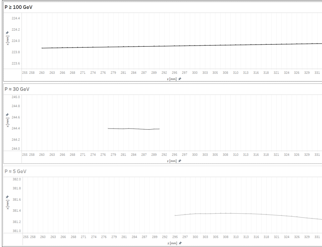
Figure 4.31: An illustration showing a visualised example of the track left by a muon ( Top ), electron ( Middle ) and hadron ( Bottom ). The scale has intentionally been altered for demonstration purposes and is not consistent.
