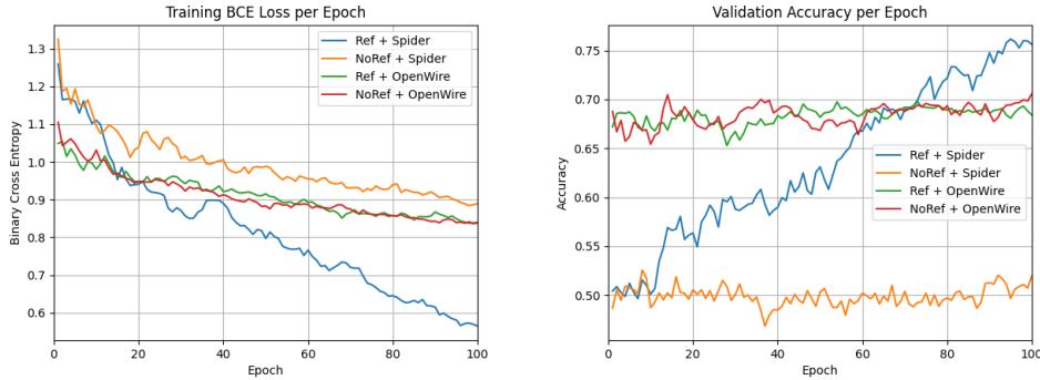
Figure 15: Training data for the four kinds of circuit structures. On the left is the training BCE computed at each epoch. On the right is the accuracy computed on the validation set at each epoch.
