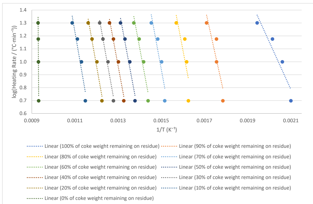
Figure A2. OFW plot for LDPE-derived coke on AXL catalyst under air atmosphere. Y-axis: \log(\text{Heating Rate} / (^{\circ}\text{C}\cdot\text{min}^{-1})) ; X-axis: 1/T \text{ (K}^{-1}\text{)} . Activation energies determined from the slopes correspond to oxidative combustion of coke fractions.
